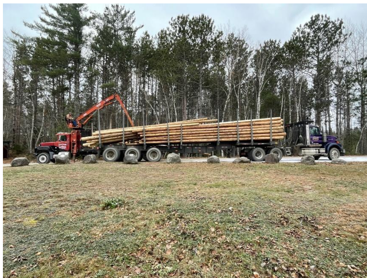
Logs being transferred from Highway Trailer to Self-Loader at Mountain View
