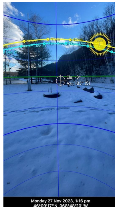
Using a Phone App to Check Winter Sun Angle and Potential Solar Charging at Matagamon
