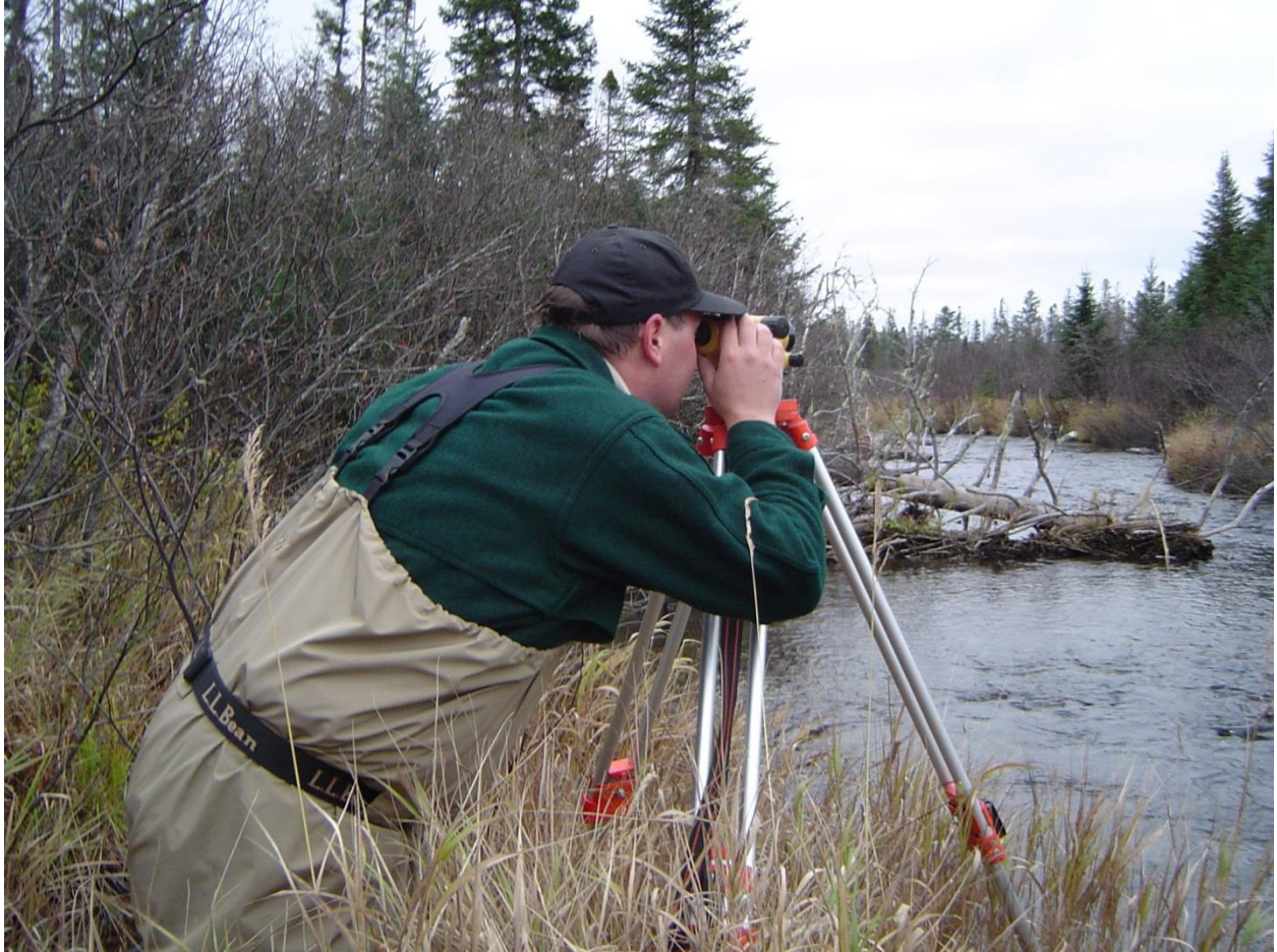
Figure 7- IFW staff using a transit level to determine slope as part of the Level II Geomorphic Survey
